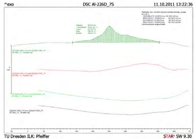
Fig. 10. DSC results of Al 226D cast plate
