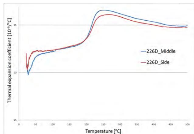
Fig. 7. Dilatometry results of Al-226D cast plate
