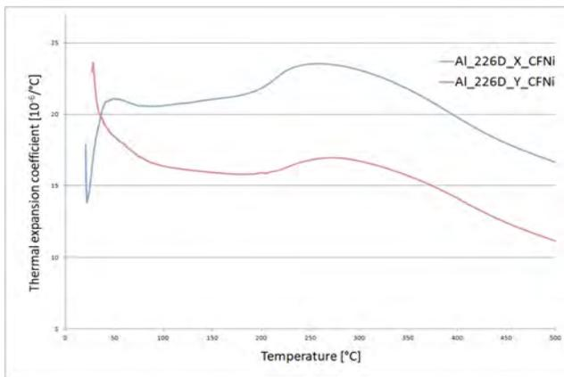
Fig. 9. Dilatometry results of 3D-CF(NiP)/AI-MMC cast plate
