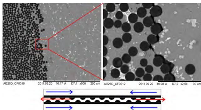
Fig. 3. Fractures at boundary between matrix and reinforcement of 3D CF/Al-MMC cast plate caused by mismatch of thermal expansion coefficient
