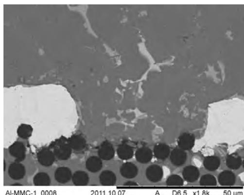
Fig. 2. Microstructure of 3D CF(NiP)/Al-MMC cast plate. Fracture occurred at boundary between matrix and reinforcement without nickel-phosphorus coating
