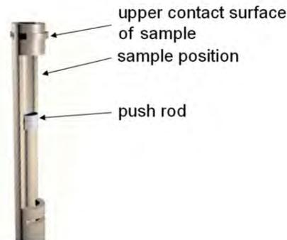
Fig. 6.  $\text{Al}_2\text{O}_3$  measuring system standard (based on LINSEIS Messgeräte GmbH)
