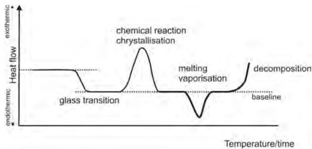
Fig. 5. Example of exo- and endothermic effects during DSC measurement [9]
