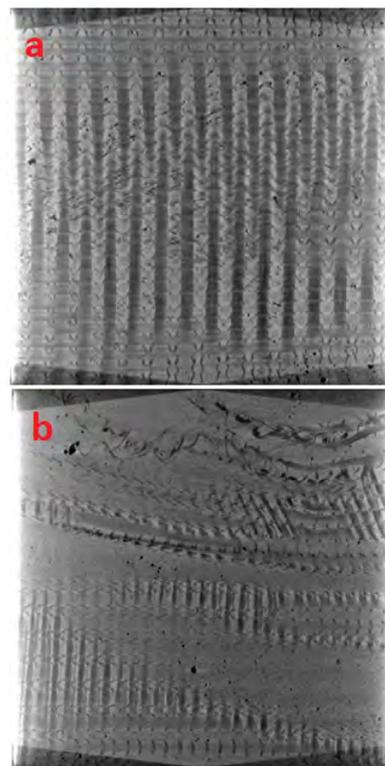
Fig. 1. Quality analysis of plates by CT: a) sufficient infiltration, b) insufficient infiltration
