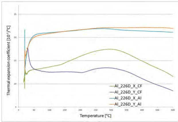
Fig. 8. Dilatometry results of 3D-CF/AI-MMC cast plate
