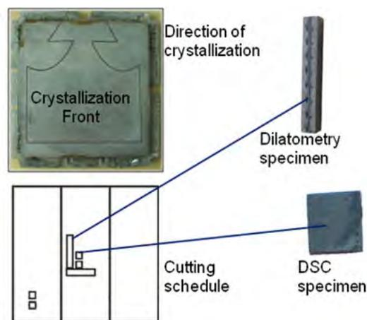
Fig. 4. Cutting lay-out of specimens
